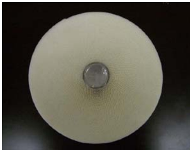
Fig. 3 Picture of PAS desiccant rotor
